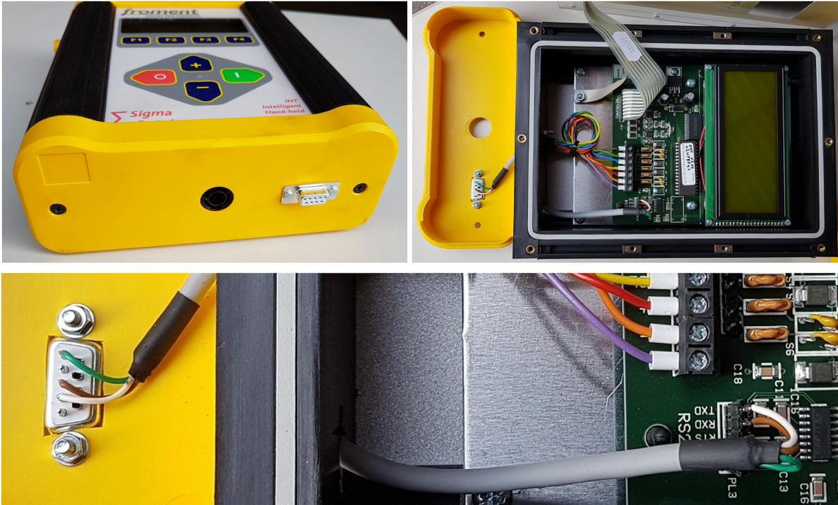
**Fig. 3. Hand-held terminal of Froment dyno with added serial-interface in evidence on its bottom side (top left); (top right) interior of hand-held terminal; (bottom) close-up view of connection between PCB and RS-232 serial interface; notice that only three pins of socket have been used**
